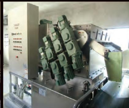
Excess Sludge at Noodle Production Plant (JD-1000)
